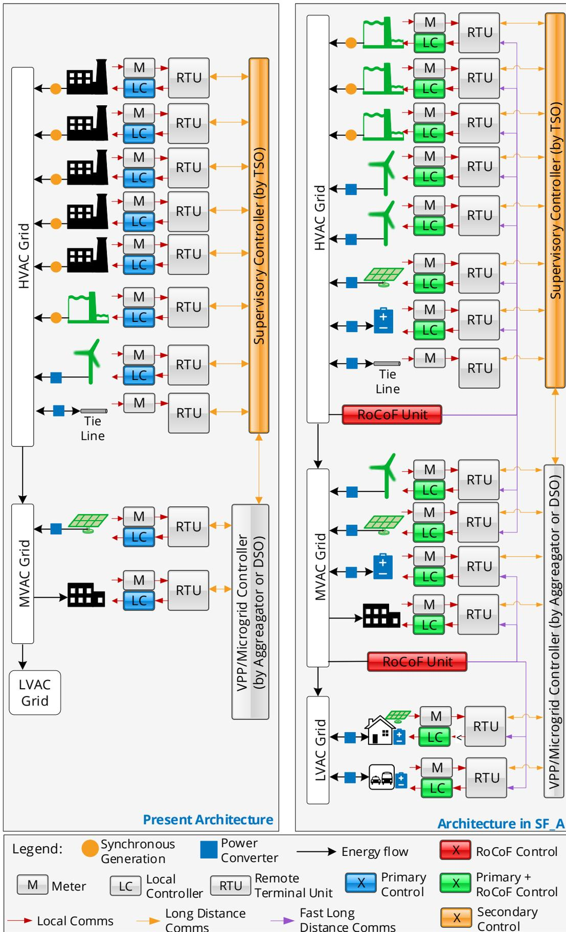
Figure 4. Frequency control architectures today and in SF\_A
