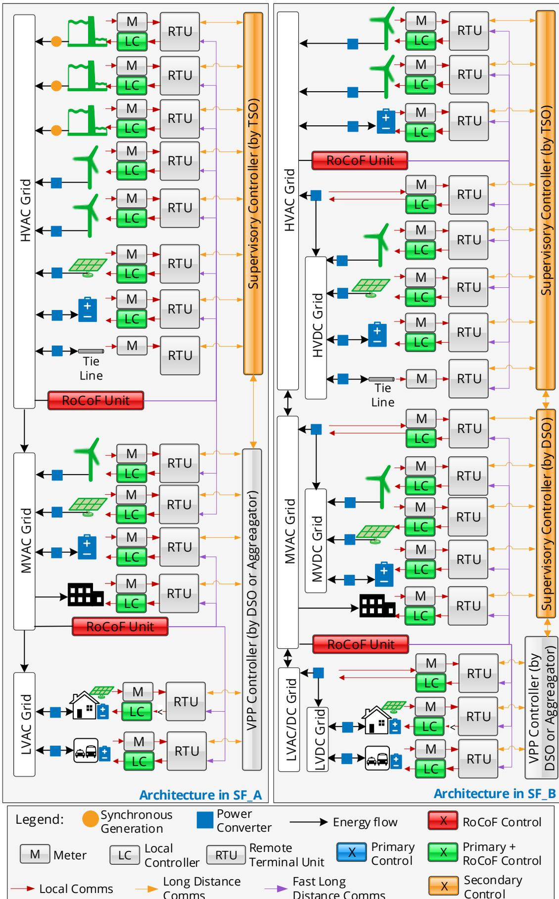
Figure 5. Frequency control architectures in SF\_A and SF\_B
