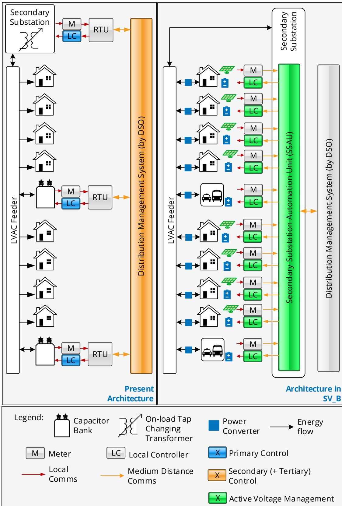
**Figure 7. Voltage control architectures today and in SV\_B**
