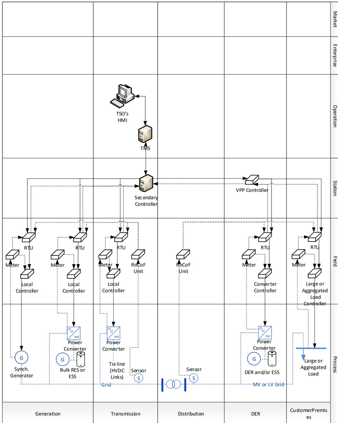
Figure 8. SGAM Component Layer for SF\_A
