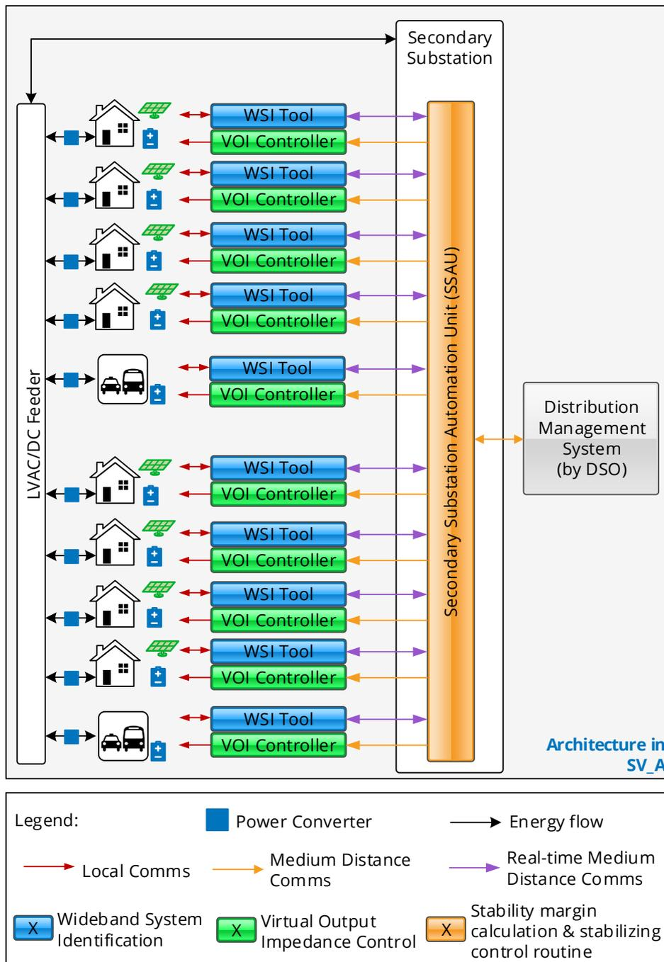
**Figure 6. Voltage control architecture in SV\_A**
