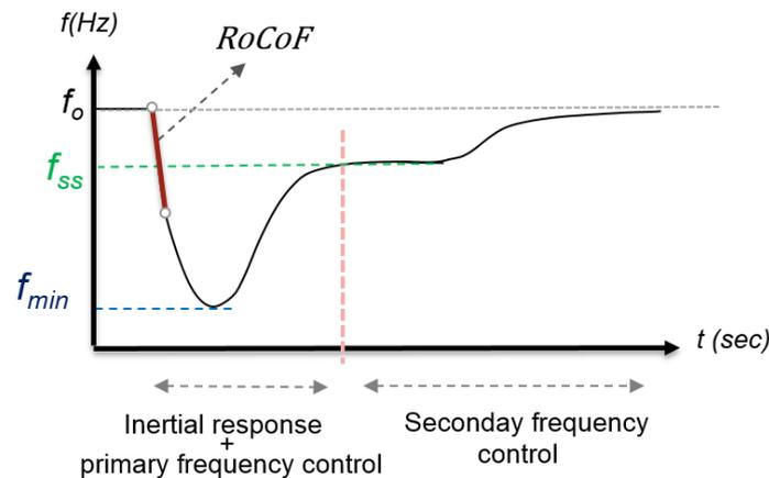
**Figure 3. Frequency deviations following a loss in power generation [Source: D1.1]**
