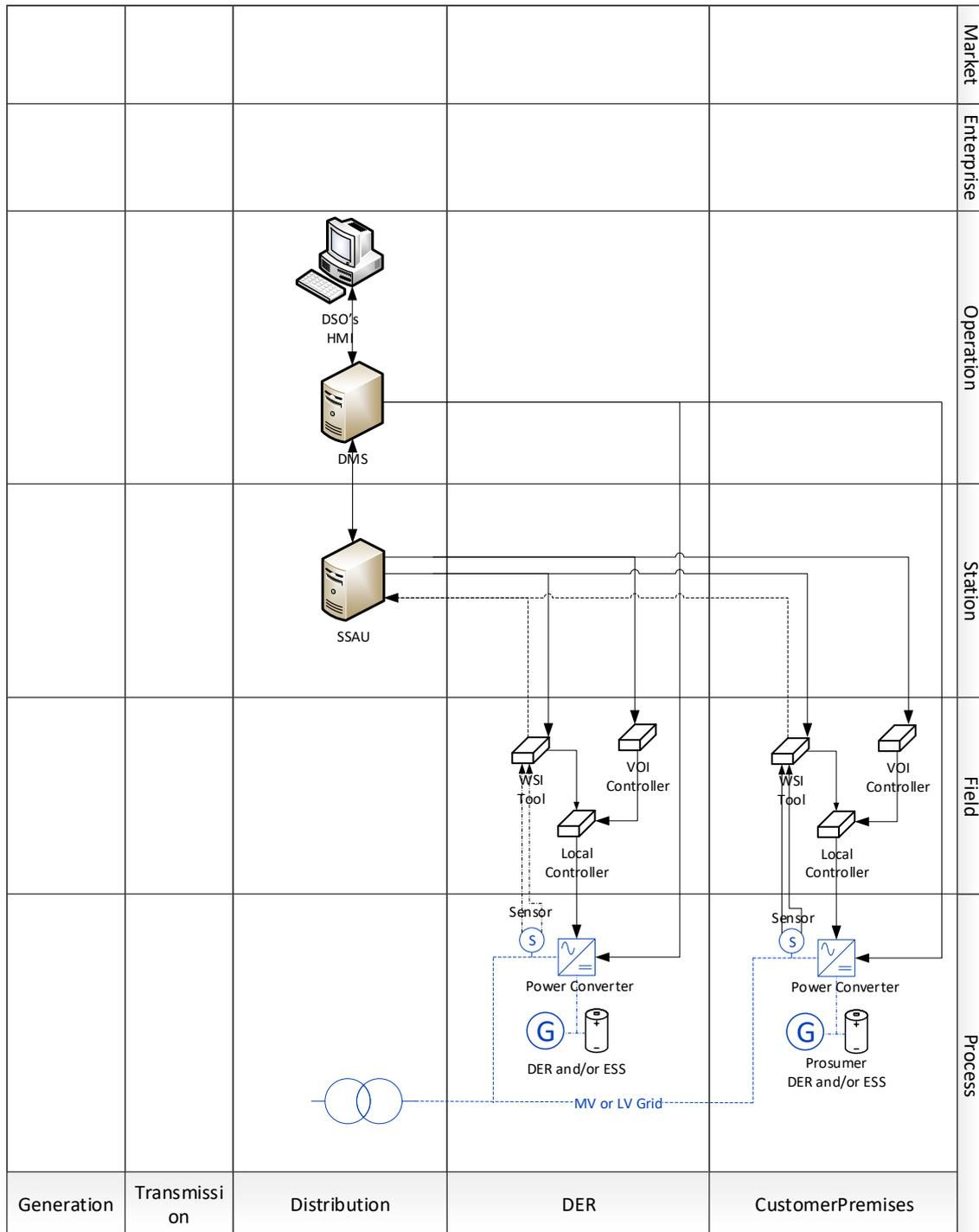
Figure 12. SGAM Component Layer for SV\_A
