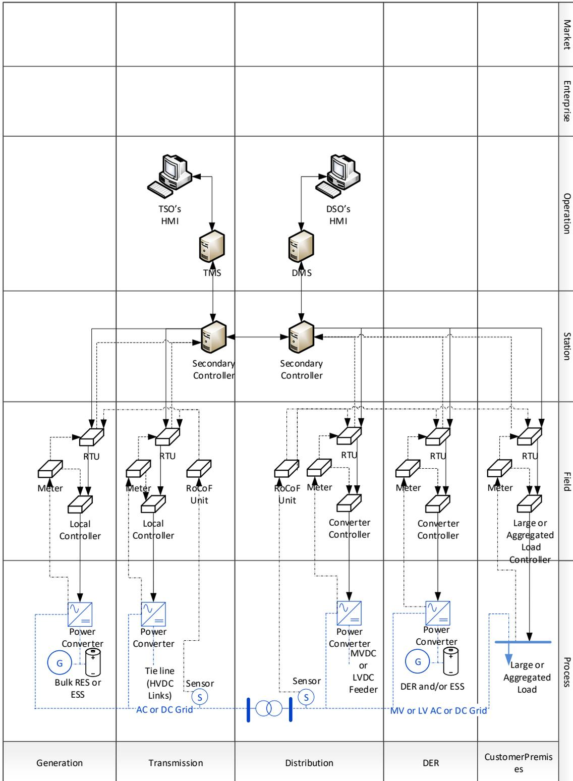
Figure 10. SGAM Component Layer of SF\_B
