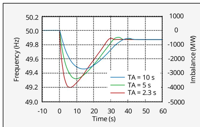
**Figure 2. Effect of inertia on the frequency deviations following a disturbance [4].**
