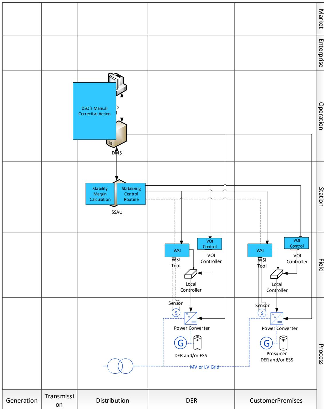
Figure 13. SGAM Function Layer for SV\_A on top of the Component Layer
