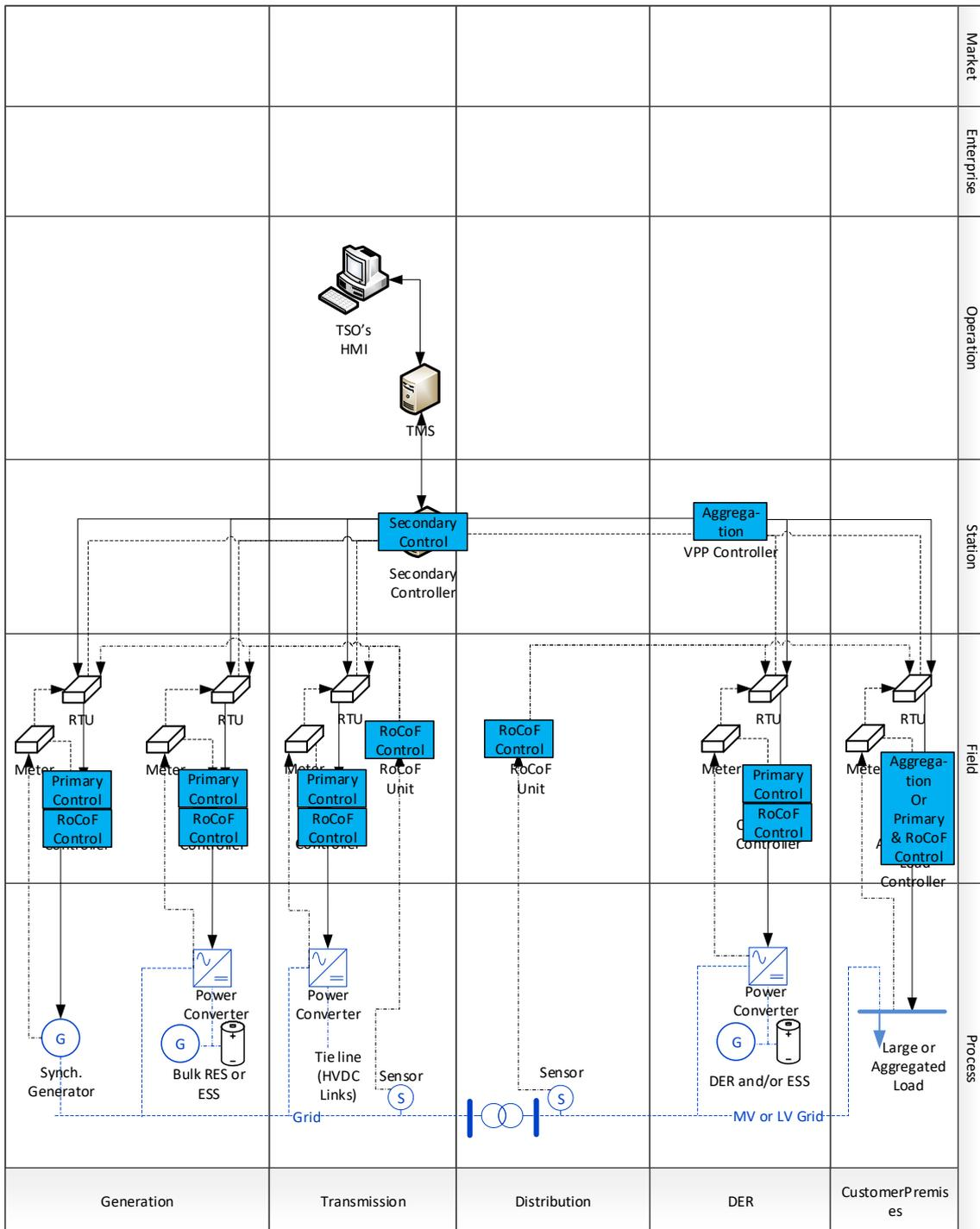
Figure 9. SGAM Function Layer for SF\_A on top of the Component Layer
