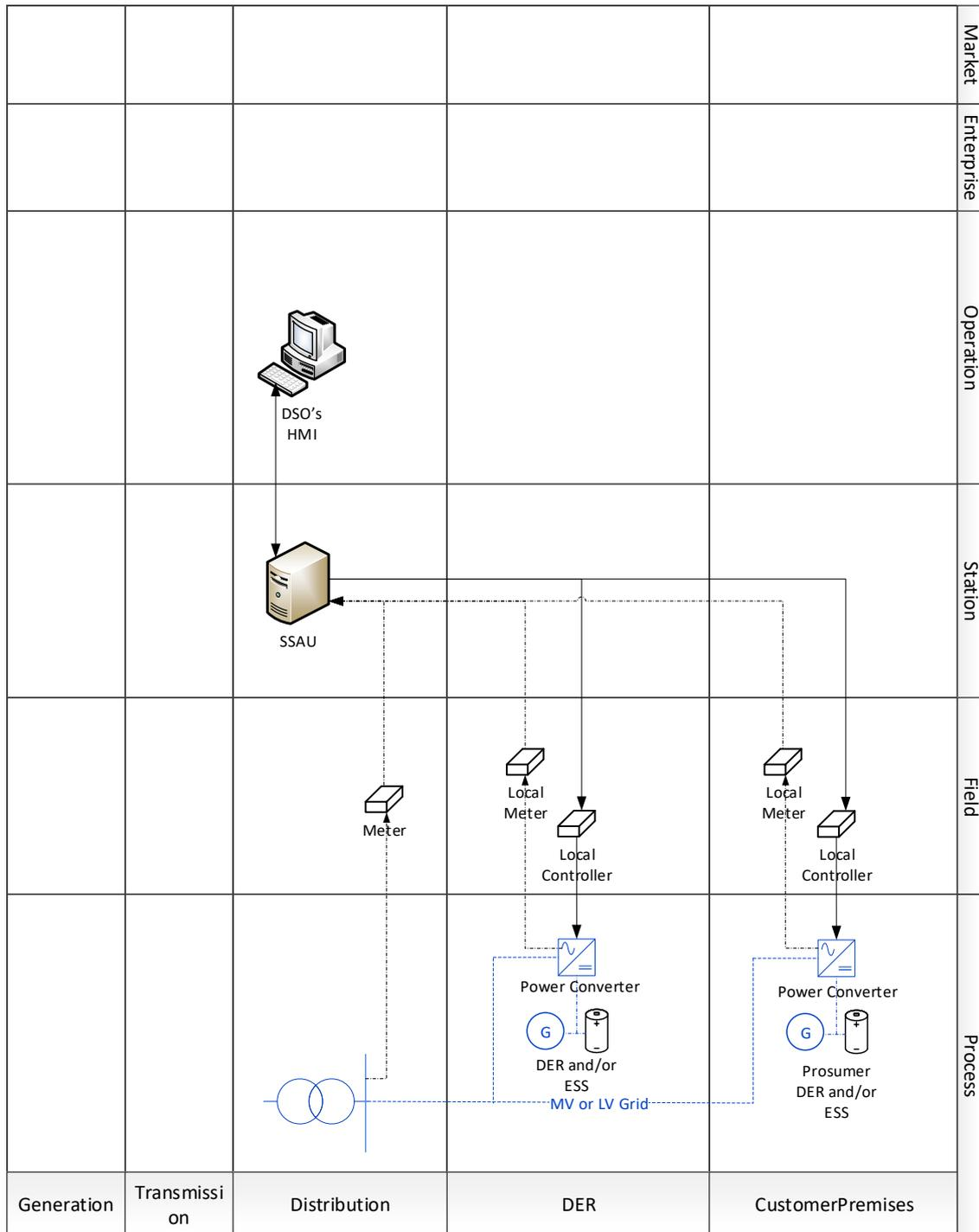
Figure 14. SGAM Component Layer for SV\_B
