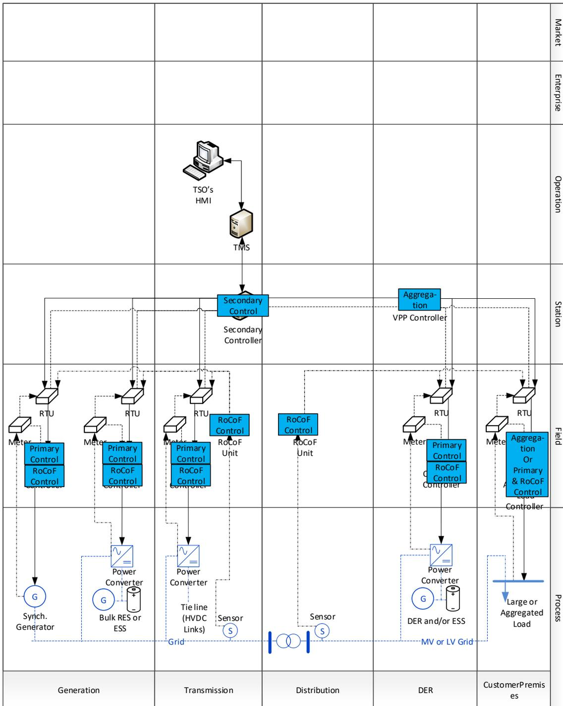
Figure 11. SGAM Function Layer for SF\_B on top of the Component Layer
